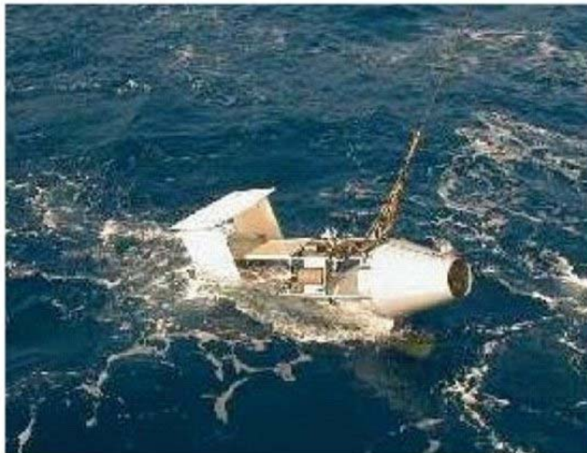
Figure 3. A modern plankton net (LHPR), being deployed from an oceanographic vessel. This net allows the collection of separate samples for different depths, simultaneously recording environmental conditions like temperature, salinity, phytoplankton (chlorophyll) concentration, etc. (Photo courtesy of the UTM, Institut de Ciències del Mar, CSIC)
